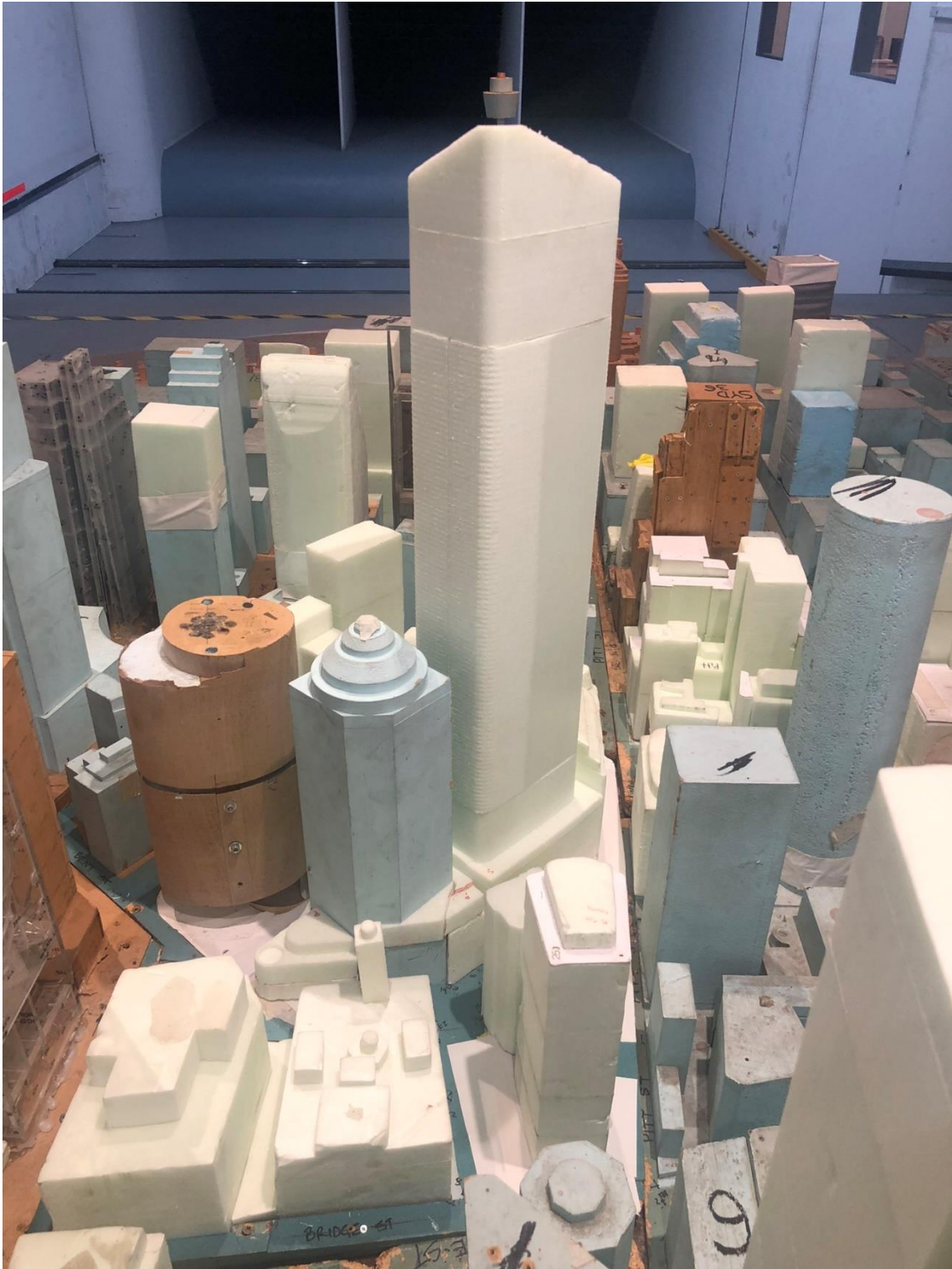
Figure 4 – View of the 1/400 scale model of the Proposed Envelope in the wind tunnel.
